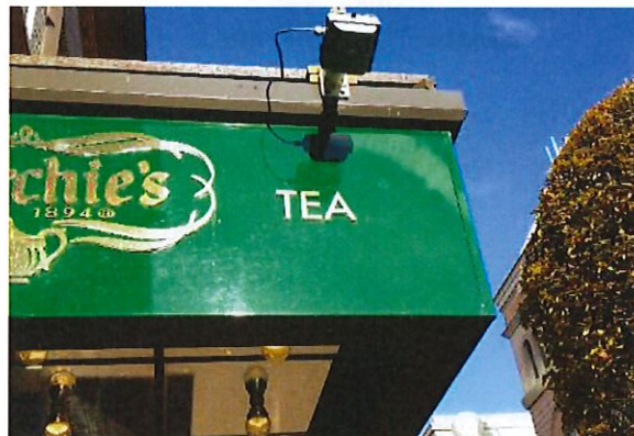
The CITIX-IR can be installed onto an awning, giving place managers insight into footfall.
