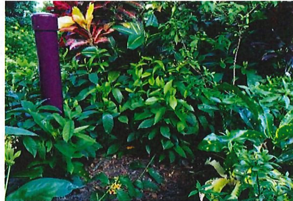
In a public park, a custom-colored, camouflaged urban post discreetly counts pedestrians passing by.
