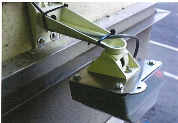
On a busy shopping street, a CITIX-IR counter is installed onto an exterior wall over the sidewalk.
